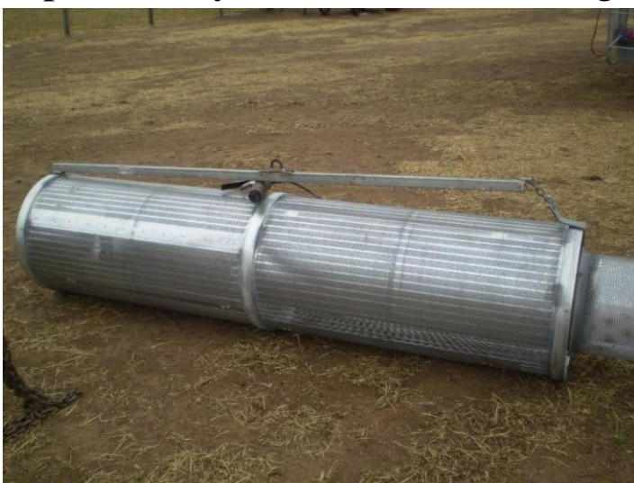
Homemade Screen lifting frame.
