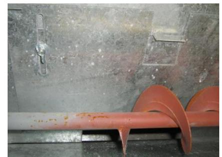
Canola/ Lupin slides are located in the inlet box of air machines only. To use these; open the width flap all the way loosen wing nuts and slide down top and bottom plates then slide top plate to approximately 15mm wide opening then tighten wing nuts to secure. The gap should be wide enough to allow pods to flow into the screens without blocking.
