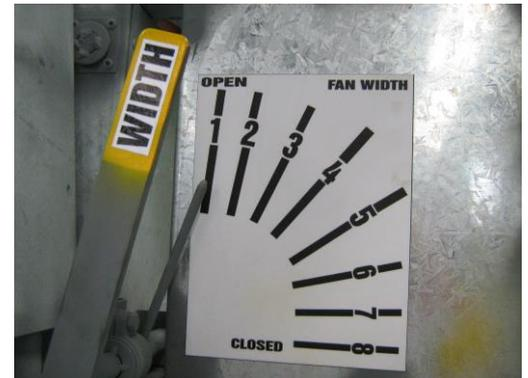
Air can be used to take off lighter material mainly in lupin or pea cleaning though is not recommended for canola. When grain is falling evenly across the width of the machine, increase the amount of air through the fall of grain by moving the air shut off handle clockwise (to the right) until good grain is near to blowing over the flap into the seconds bag. More very light material can be blown off by increasing the amount of air used and adjusting the flap to retain good grain blown further.
